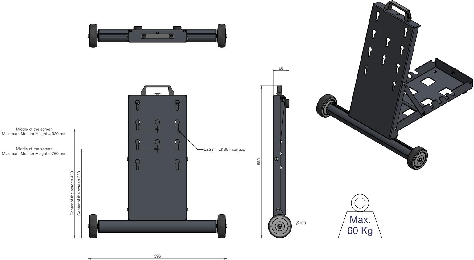
The Podium stand can be positioned in 5 angles ranging from 35 up to 75 This product must be combined with an Audipack UFPRO monitor bracket
